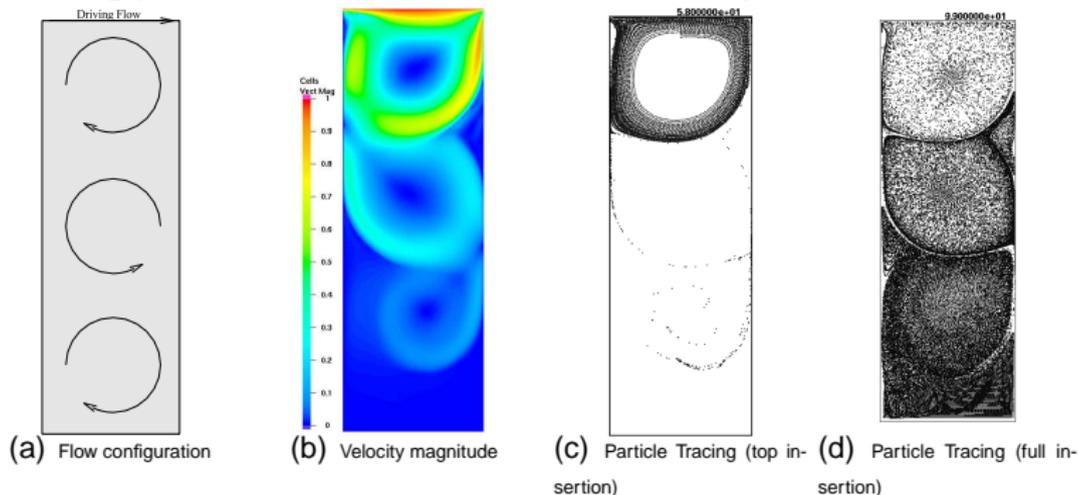
Figure: Snapshots for 'Driven cavity'
