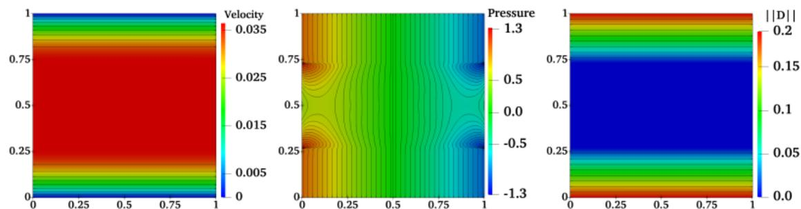
Figure: Visualization of the velocity contours, pressure and  $\|\mathbf{D}(\mathbf{u})\|$  for the non-regularized Bingham fluid flow in a channel with  $\tau_s = 0.23$  at refinement level  $L=5$  ( $h_x = 1/32$ ,  $h_y = 1/96$ ).
