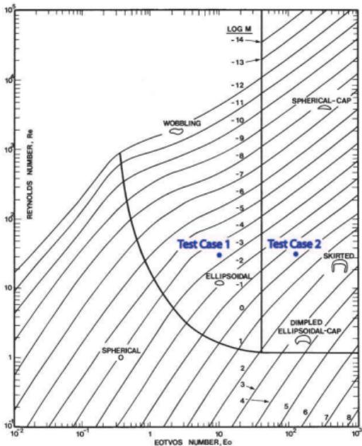
Figure: Shape regimes for bubbles and drops in unhindered gravitational motion through liquids [Clift et al., Bubbles, Drops and Particles (1978)]
