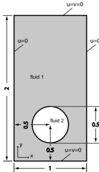
Figure: Initial configuration and boundary conditions for the test cases
