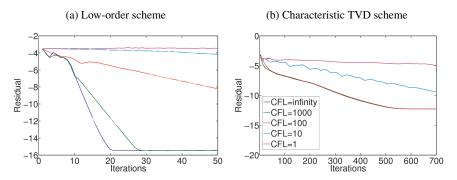
Fig. 11 NACA 0012 airfoil: convergence history for various CFL numbers on mesh level 2.
