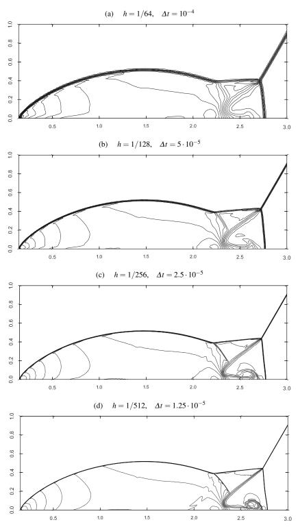
**Fig. 6** Double Mach reflection: isodensity contours at T = 0.2; unsafe FCT<sup>*Roe*</sup>,  $\alpha_{ij}(\rho, p)$ .
