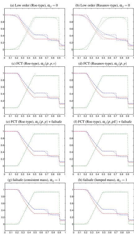
Fig. 1 Shock tube problem:  $h = 10^{-2}$ ,  $\Delta t = 10^{-3}$ . Snapshots of the density (blue), velocity (green), and pressure (red) distribution at the final time T = 0.231.
