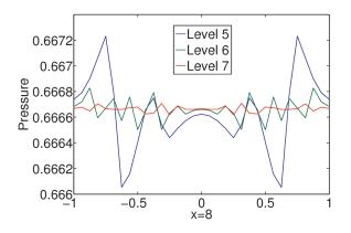
Fig. 13 Converging-diverging nozzle: exit pressure distribution.
