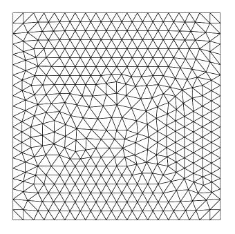
Fig. 2 Radially symmetric Riemann problem: coarse mesh, 824 triangles, 453 vertices.
