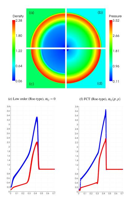
Fig. 4 Radially symmetric Riemann problem: density (red) and pressure (blue) at T = 0.13.
