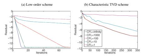
Fig. 9 GAMM channel: convergence history for various CFL numbers on mesh level 4.
