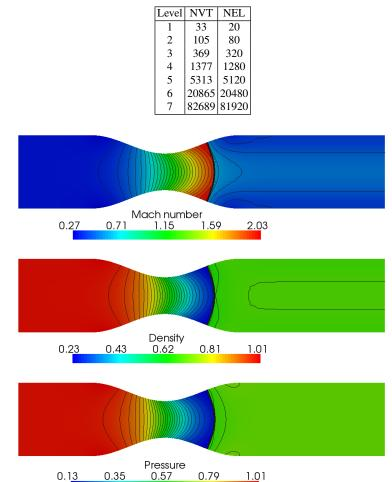
Table 10 Converging-diverging nozzle: mesh properties.
