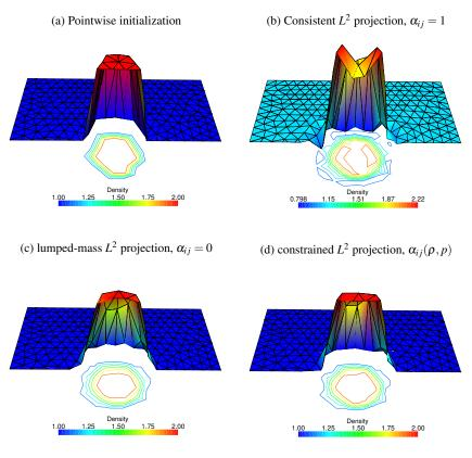
Fig. 3 Radially symmetric Riemann problem: initial density  $\rho_h^0$  on the coarse mesh.
