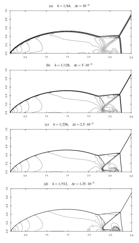
**Fig. 7** Double Mach reflection: isodensity contours at T = 0.2; unsafe FCT<sup>*Roe*</sup>,  $\alpha_{ij}(\rho, \rho E)$ .
