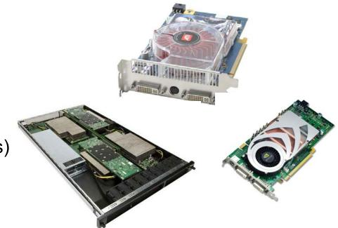
GPU (NVIDIA GTX 285): 240 cores @ 1.476 GHz, 1.242 GHz memory bus (160 GB/s)  $\approx$  1.06 TFLOP/s
