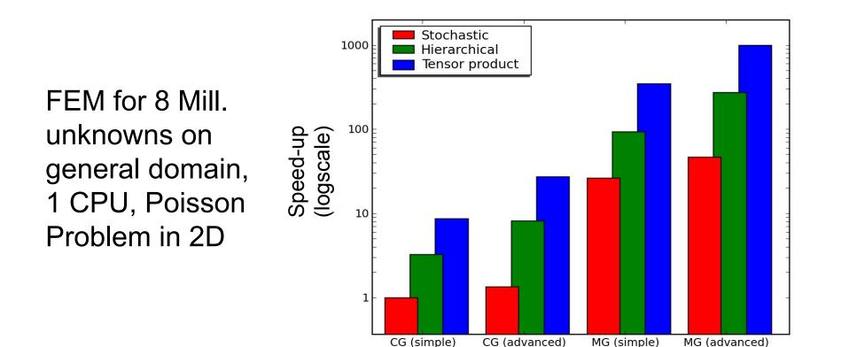
Dramatic improvement (factor 1000) due to better Numerics AND better data structures/ algorithms on 1 CPU **FEAST** – Realization of HwoN
