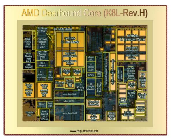
**CPUs** devote most of the transistors to caches and data movement for general purpose applications
