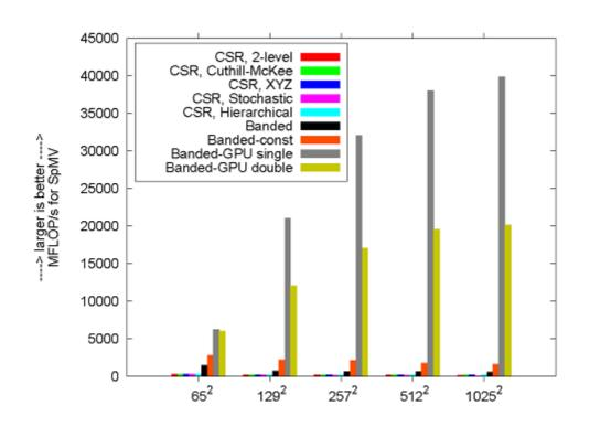
40 GFLOP/s, 140 GB/s with CUDA on GeForce GTX 280 'only' 13 GFLOP/s on 8800 GTX (90 GB/s peak)
