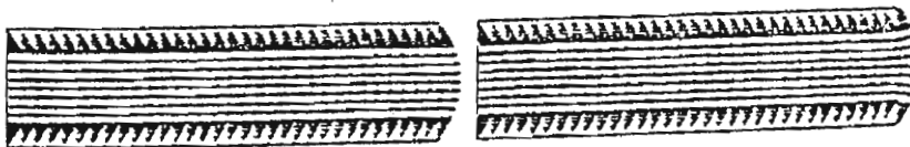
Figure 10. Vector plots of pipe flow at Re = 50 with an artificial outflow boundary. The computation on the left is based on the standard variational formulation (8). The computation on the right is made similarly but with the term v(\nabla u, \nabla \varphi) in (8) replaced by v(Du, D\varphi) , where D is the deformation tensor
