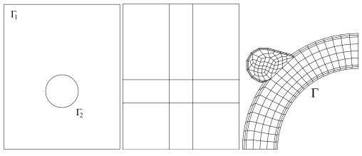
(a) geometry of the CIRCLE (b) coarse grid of the CIRCLE (c) coarse grid of the BLOOD setup setup
