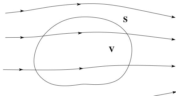
fixed CV of a finite size
